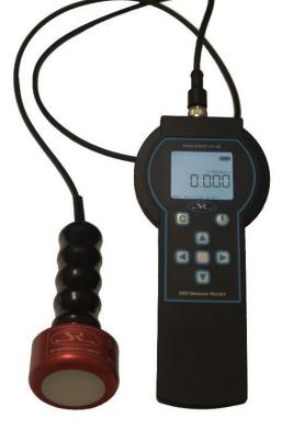
Radome GO / NO GO, with variable sound level indicator & 3 x density settings (honeycomb, foam & solid)
