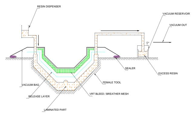
Accelerated curing can proceed once impregnation has been completed using either ovens, autoclaves or other heat sources.
